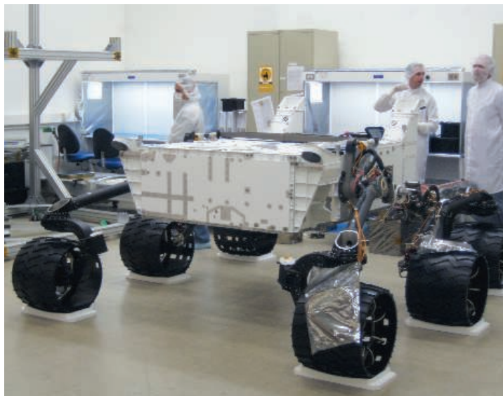
Let's roll. Wheels have been fitted to NASA's Mars Science Laboratory (MSL) rover, which is being assembled at NASA's Jet Propulsion Laboratory, Pasadena, California. The rover has a ground clearance of about 60 cm, or 2 feet, and is about the size of a small automobile.
